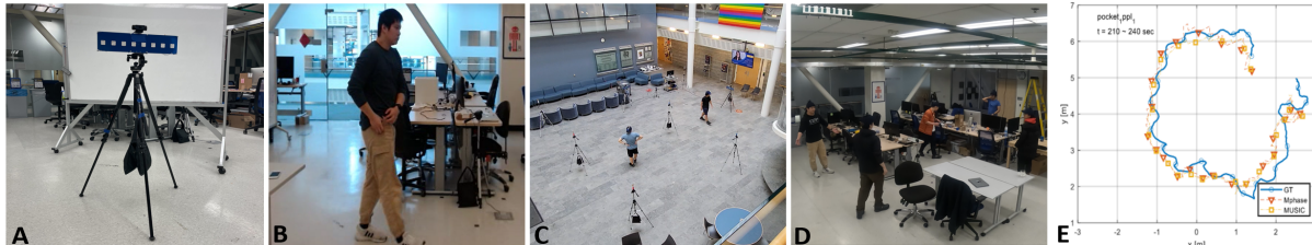
Fig. 1. This work uses an 8-element switched antenna array with a single chain receiver shown in (a) to estimate the AoA of commodity BLE devices. A phone transmitting BLE packets is carried in the user's pocket shown in (b), while the user walks around the space. A technical evaluation in a low-multipath lobby environment (c) and a real-world usage evaluation with multiple users are conducted. The 2D trace of the user shown in (e) combines the AoA estimations from two antenna arrays.
