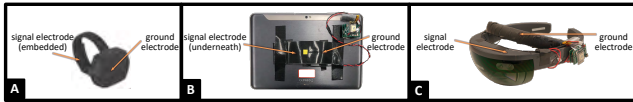
Figure 4: User-worn BCC device options. A: Light-weight BCC wristband. B: BCC-Tablet integration. C: BCC-HoloLens integration.
