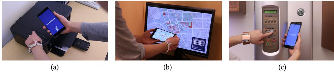
Fig. 10. Images of the three demo applications developed using the EM-Comm technology. They include (a) pairing, trouble shooting, and printing from a Mobile phone, (b) grabbing a map & directions from a public LCD display and sending them to the users smart phone, and (c) launching virtual tool tips of button functionality on a coffee machine
