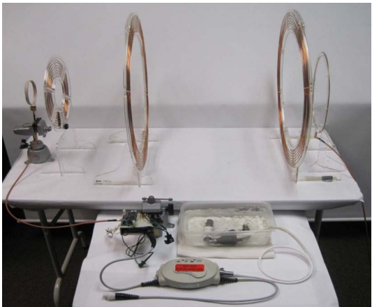
Fig. 17. Configuration for the axial VAD experiment showing the VAD being wirelessly powered via the FREE-D system, which is connected to the RF-dc rectifier and dc-dc regulator circuit and the HeartMate II System Controller.
