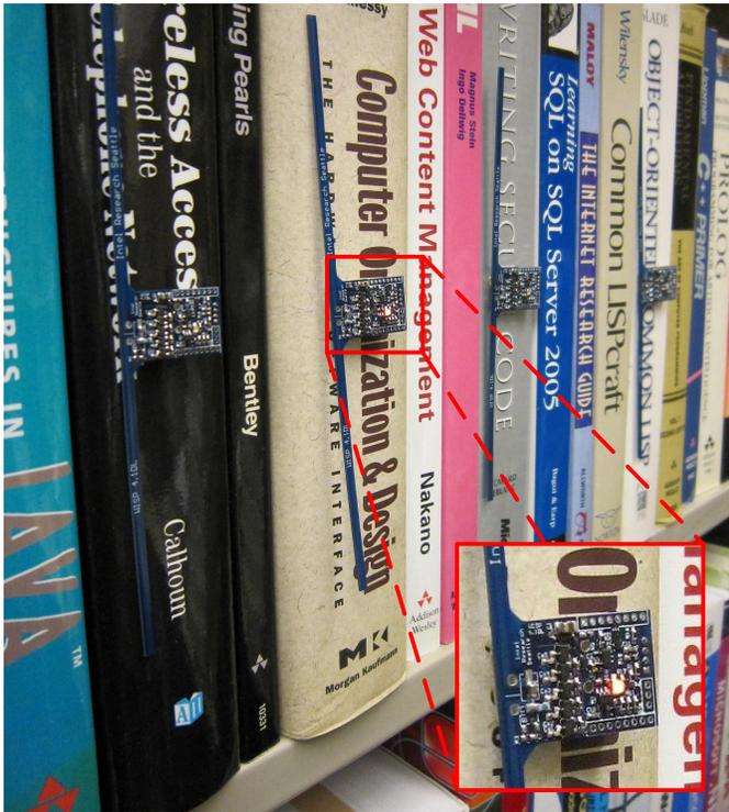
Fig. 2. Demonstration of an enhanced passive RFID tag flashing its LED when commanded to by an RFID reader. The WISP 4.1 platform is used for prototyping. The pop out shows a detailed view of the LED flashing, which is clearly visible to spectators at distances over 10 meters.
