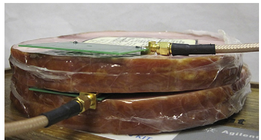
Fig. 23. PCB resonators with ham in physical contact with the receive resonator.
