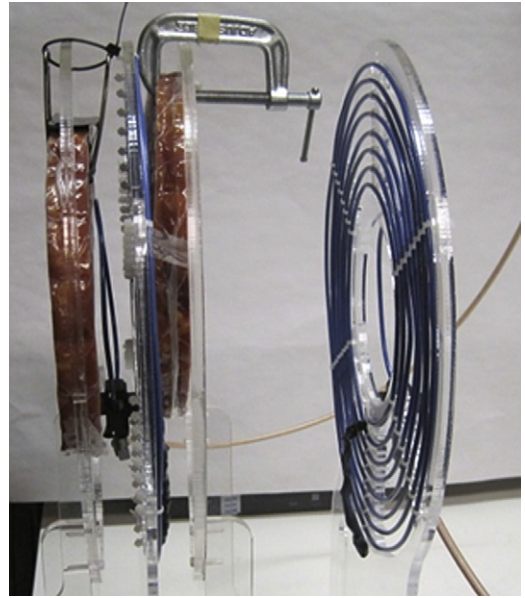
Fig. 22. Insulated copper resonators with ham in physical contact with the receive resonator.
