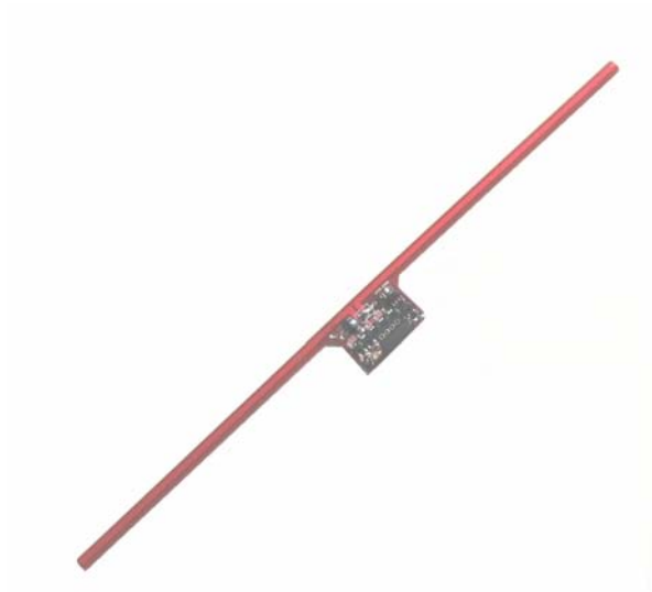
Fig. 3. WISP photograph. This WISP includes a 3 axis accelerometer.
